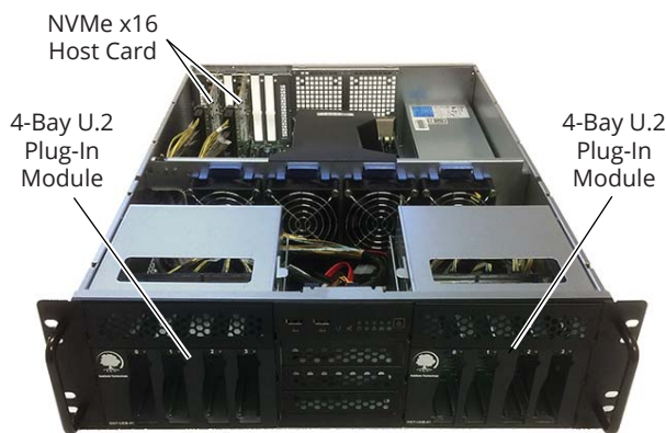
3U Rackmount Appliance with Two 4-Bay Single/Dual-Port NVMe U.2 Plug-In Modules Installed
